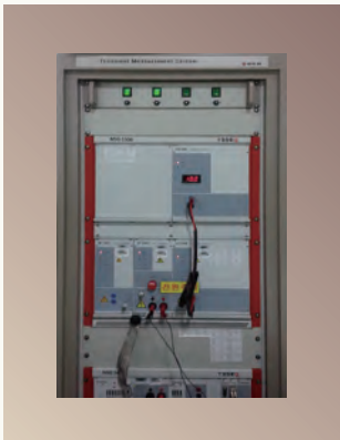
Transient test system (External)
